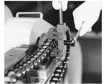
Fig. 5 How to cut a chain using a chain breaker
