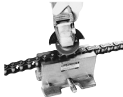
Fig. 2 Grinding the pin ends
