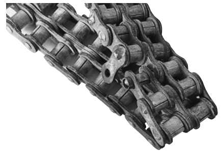
Fig. 31 Corrosion of stainless steel roller chain
