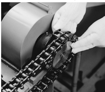
Fig. 8 Connecting on a sprocket
