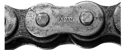
Fig. 32. Hydrogen embrittlement cracking
