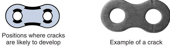
Fig. 23 Cracks on the link plates
